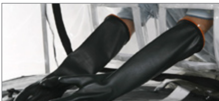
Conduit sleeves – removable and replaceable gloves
